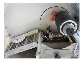
The patented cassette type press-out system (see the picture above) is at the core of the Deblimatic<sup>®</sup> deblistering machine. The machine comes with two cassettes. Additional cassettes can be ordered separately.
