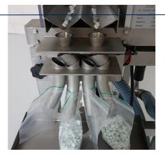
The above photograph shows the counting and automatic filling unit of the Deblimatic<sup>®</sup> L16. The number of medication pills, tablets or capsules that have to be filled in each of the pouches can be programmed very easily. Of course, the counted medication can also be filled in jars instead of pouches.
