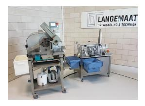
One Deboxmatic L17 machine can feed at least one automatic Deblimatic L16 or Deblimatic A19 deblistering machine and depending on the number of blisters per box even two Deblimatics. In the above picture the blisters from the Deboxmatic (on the right) can be fed immediately to the Deblimatic L16 (on the left).
