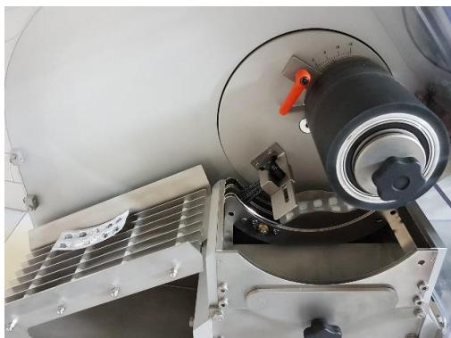
The patented cassette type press-out system (see the picture above) is at the core of the Deblimatic® deblistering machine. The machine comes with two cassettes. Additional cassettes can be ordered separately.
