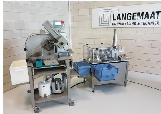
One Deboxmatic L17 machine can feed at least one automatic Deblimatic L16 or Deblimatic A19 deblistering machine and depending on the number of blisters per box even two Deblimatics. In the above picture the blisters from the Deboxmatic (on the right) can be fed immediately to the Deblimatic L16 (on the left).
